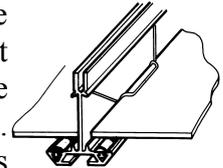
Bar Capping should be fitted 'as you go along'. You need access to the top of each roof cap to screw into position, so you will need to poke your head up in the next bay along to enable safe fixing.
