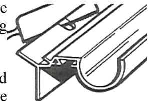
5. Slide the 2 bolts into the bolt slot facing inwards i.e. the alternative bolt slot of the corner bars to the holes in the cill and eave/gutter. Put a nut on and finger tip tighten. Do the same with the left hand roof corner bar, having first inserted 3 bolts into each bolt slot. (Don't forget to ensure that the "R" is at the ridge and **not** the eave). Do the same with the other side and roof corner bars.
