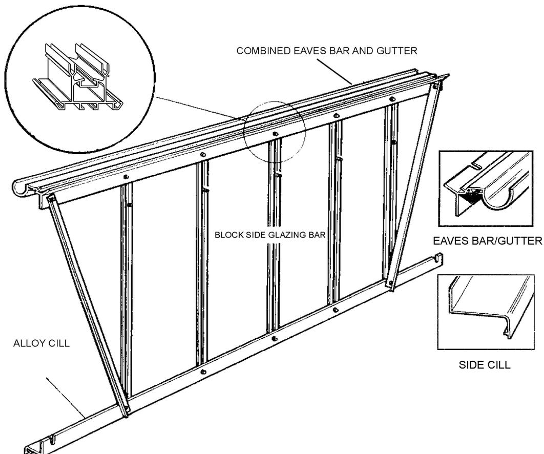
1. Lay out the pieces on the ground as though you were standing inside the greenhouse i.e. with the gutter and cill facing downwards and the inside bolt channel of the glazing bar upwards (beading channels downwards). **(Key point)**. Slide the glazing beading into the 'V' grooves of the glazing bars, taking care not to stretch the material. Trim off any surplus level with the ends of the glazing bar. Note: the beading may contract and slide down the bar. Allow for this before trimming.
