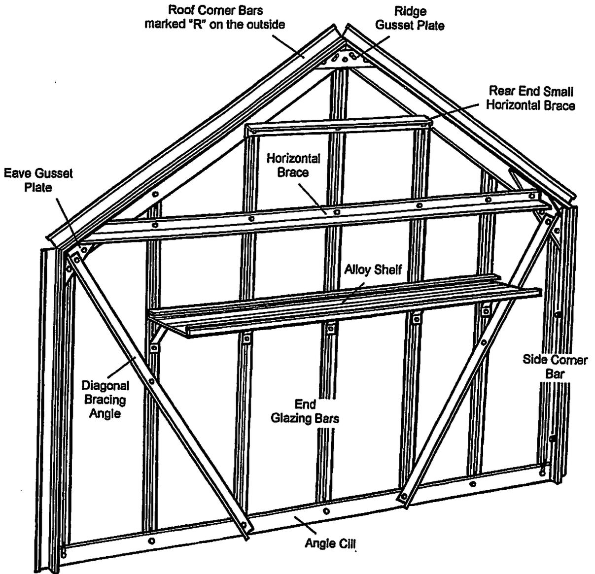
7. Do exactly the same with the other roof corner bar ensuring that the two bars are pressed tight up together behind the ridge gusset plate.
