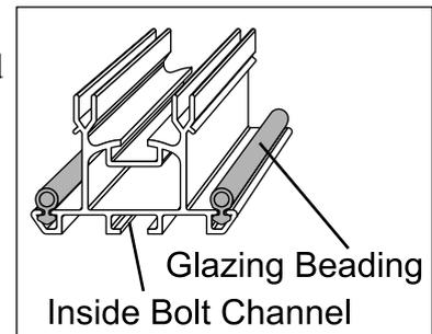
2. Slide 3 bolts into each glazing bar (insert an extra two bolts into the bars that the louvre vent will attach to **(Key point)**). The middle bolt will be used later to attach the cantilever tee bars.
