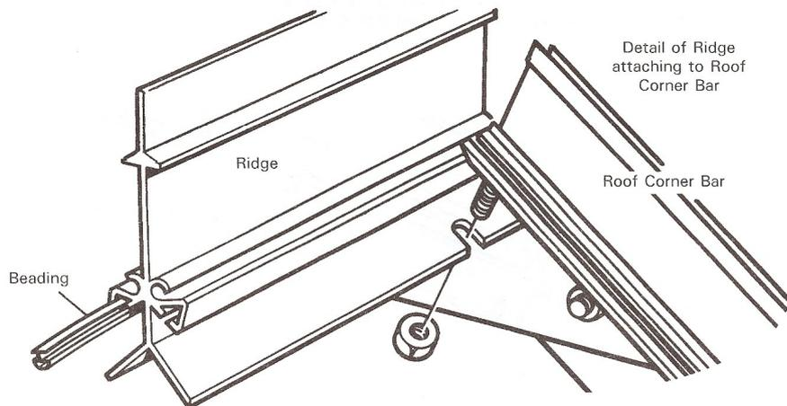
6. The ridge bar is fitted next, but first you must thread the glazing beading into the 2 grooves on the ridge. **(Key point)**. Lift the ridge bar up to the apex and standing on a pair of sturdy
