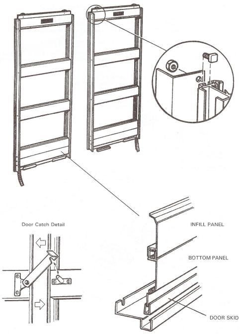
illustrated. You will need to drill four 5mm holes in the relevant door panels and attach the catch and keep, utilising the small nuts and bolts provided. Position the keep so that the catch fits snugly and the doors close tightly.
