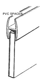
The glass to fit along the front (under the gutter) is required to be longer than the glass supplied. To overcome this, you will find a number of PVC spacer bars inside the packet of glass delivered (full sheet toughened glass only). This spacer must be fitted to the top of the front pane before the glass is installed to the front assembly. Please see diagram below
