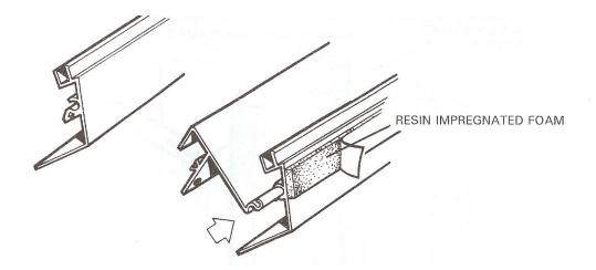
The vent slam can now be fitted to the roof bars just underneath the bottom rail of the vent. The ends of the slam bar are cut out to go round the profile of the roof glazing bar. Secure the slam bar with the two bolts that were inserted when you fitted the bottom of the roof bars to the eave.
