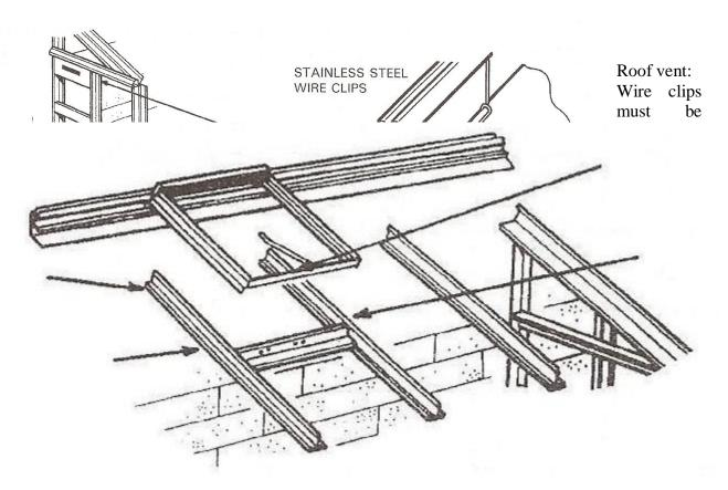
used on the panes of glass either side of the vent. The wire clips are only necessary on the sides of the glass nearest to the vent. This is because the vent side rails overlap the roof glazing bars. See diagram below.
