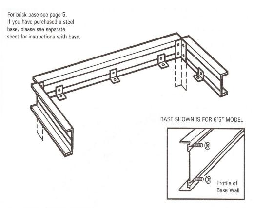
Alloy base (when fitted to soil floor).
