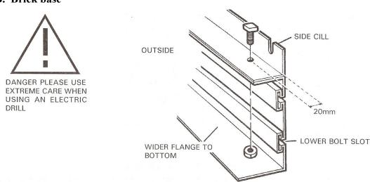
There are a number of small angle brackets in the pack of fittings; these are to be bolted onto the upright glazing bars at the point where the cills are attached to them. Before bolting them to the frame, first mark the brickwork where the holes are to be drilled. Drill the holes with a masonry bit and insert the plastic plug. Secure the small angle to the uprights and screw through the hole in the angle into the plug as illustrated.
