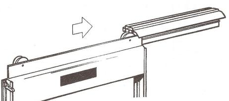
screw and secure. This will prevent the door track from any sagging when the door is in the open position.
